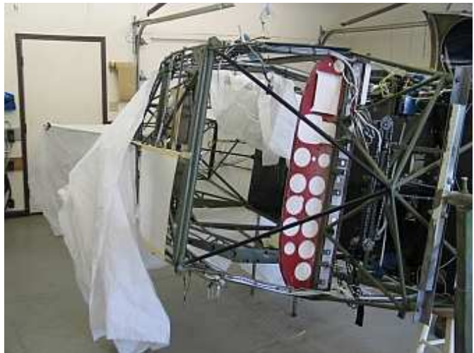
The fuselage "sock" is loosely pulled over the airframe.
